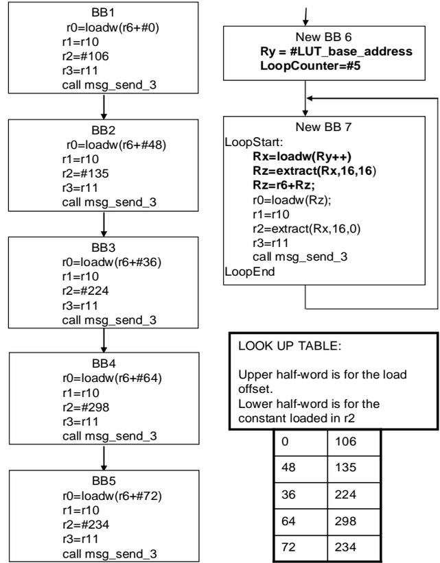
(a) CFG before code size optimization      (b) CFG after code size optimization
