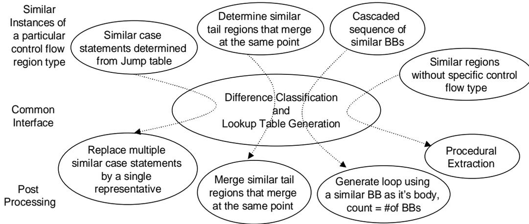
Figure 6: Overall infrastructure of code size optimization using difference classification and LUT generation.
