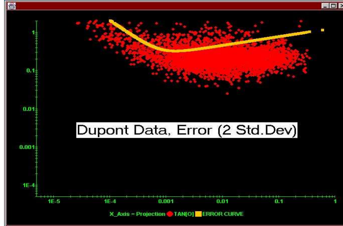
Figure 13: Dupont's Data \tan(\theta) vs. Projection (Delimiter value = 2 * \sigma )
