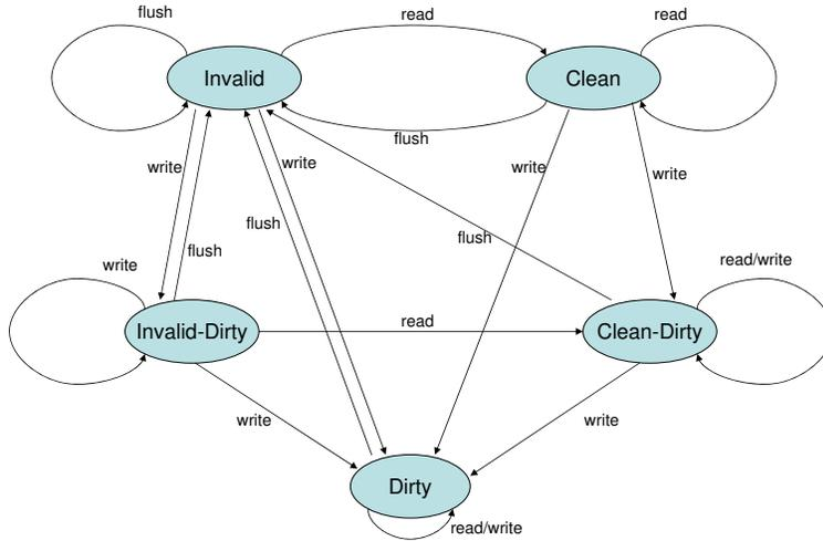
Figure 2: State transition diagram for the cache protocol of *ModelLF*.
