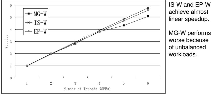
Figure 3: Speedup as a function of the number of SPEs under *ModelLF* cache protocol.
