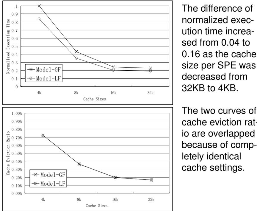
Figure 5: Trends of execution time and cache eviction ratio for MG-W on various cache sizes.
