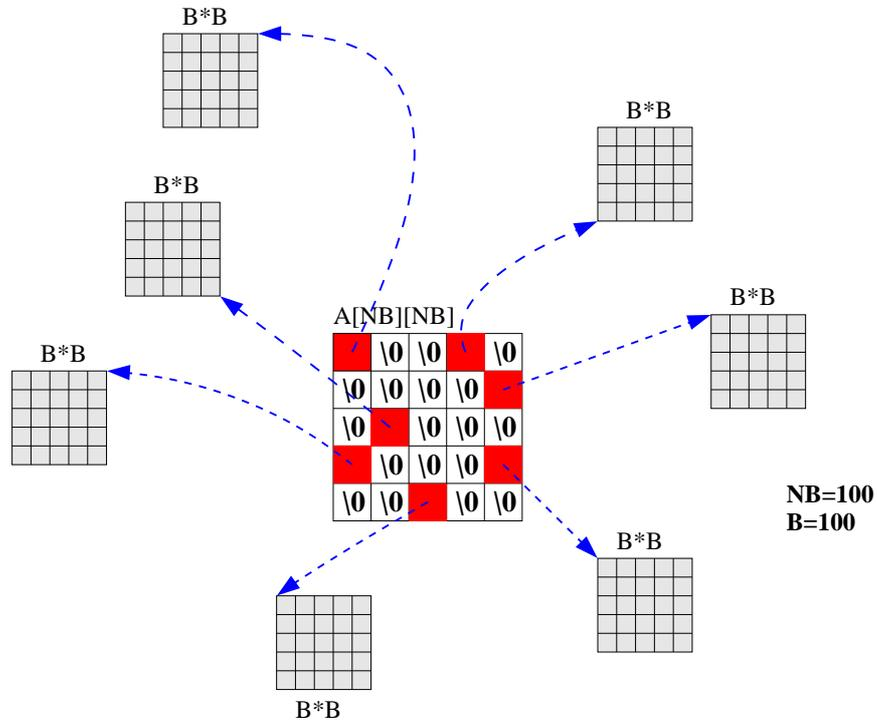
**Figure 4.4:** The 2-level hierarchical data structure used in *sparseLU* code
