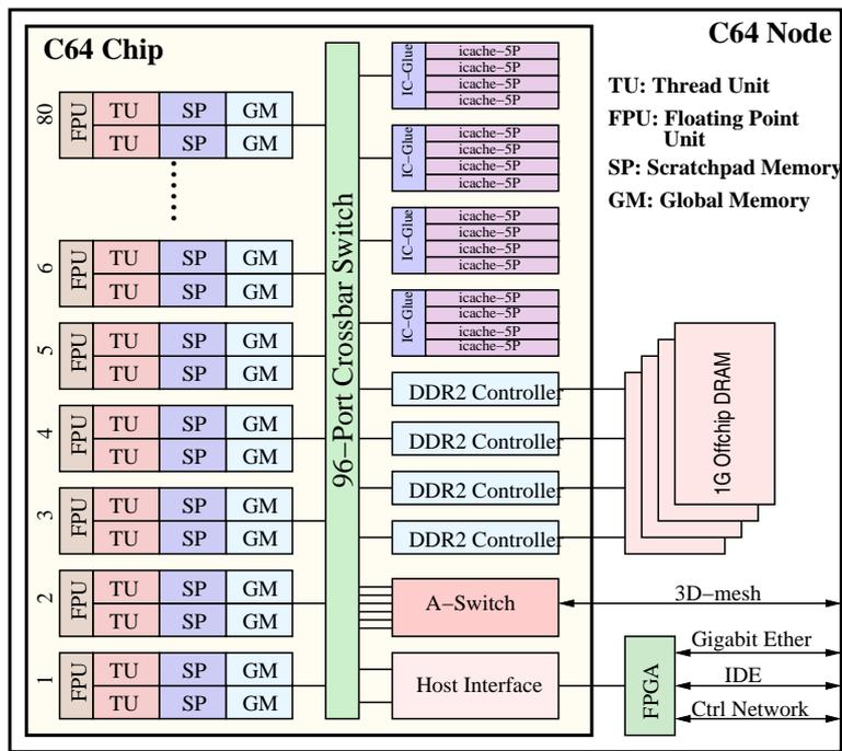
**Figure 1.1:** The IBM Cyclops-64 Manycore Processor
