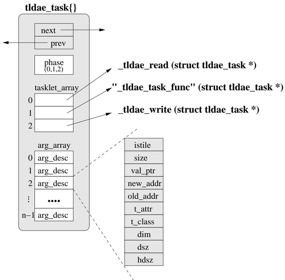
**Figure 4.10:** Diagram of the tldae\_task{} structure
