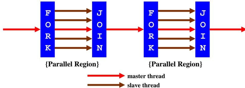
**Figure 1.3:** OpenMP Fork-Join Execution Model
