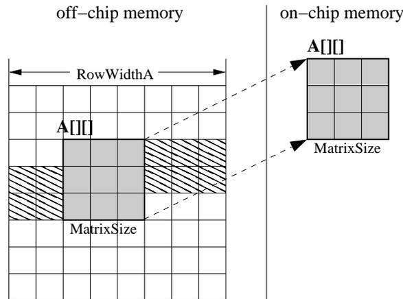
(b) Diagram of embedded matrix A
