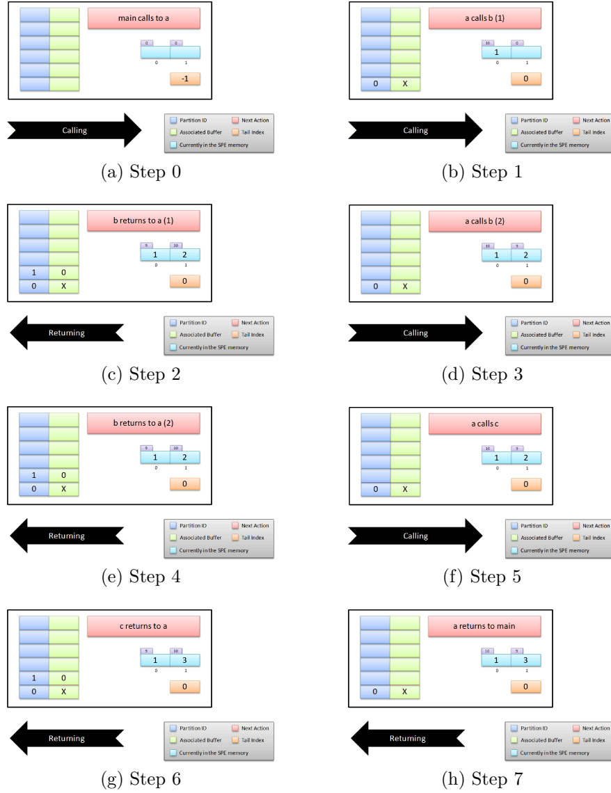
Figure 5.4: States of each of the partition manager components across the function calls provided by source code in listing 5.2 using the LRU replacement policy
