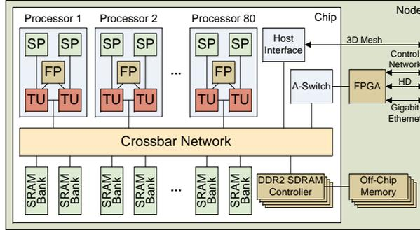
Figure 1: The architecture of a Cyclops-64 node.
